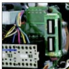
Counter for operating hours and starts
