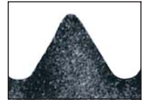
Modified thread: Note stress relieving radii in this unretouched photo enlargement of the supabuckle.
